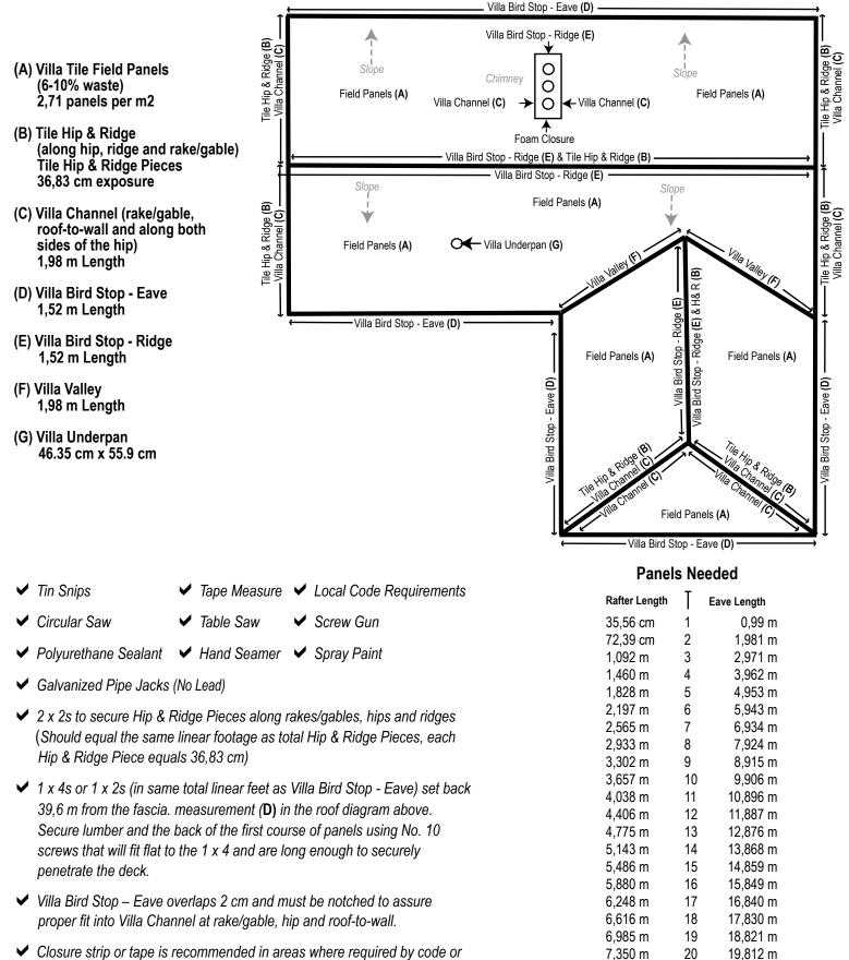
Closure strip or tape is recommended in areas where required by code or warranted by weather conditions.
