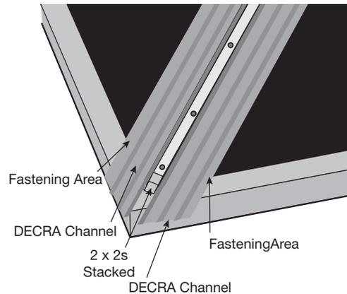
**DECRA Valley:** Install DECRA Valley or standard concrete valley metal (with same specifications as DECRA Valley) along all valleys. All valley metal should be minimum 26 gauge pre-finished aluminum-zinc alloy coated steel. Valley metal should be a minimum 16" wide, with a minimum center upstand of 3-1/4". In new construction, the metal valley flashing must have one layer of Type 30 felt underlayment, 36" wide or ice & water shield underneath as required by local building code.
