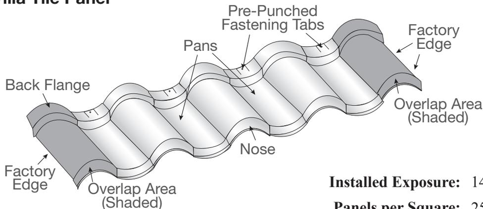
**Installed Exposure:** 14-1/2" x 39-1/2"
