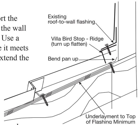
Fasten through the roof-to-wall flashing, Villa Bird Stop - Ridge and into the high point of the barrel on the panel (see diagram above right).
