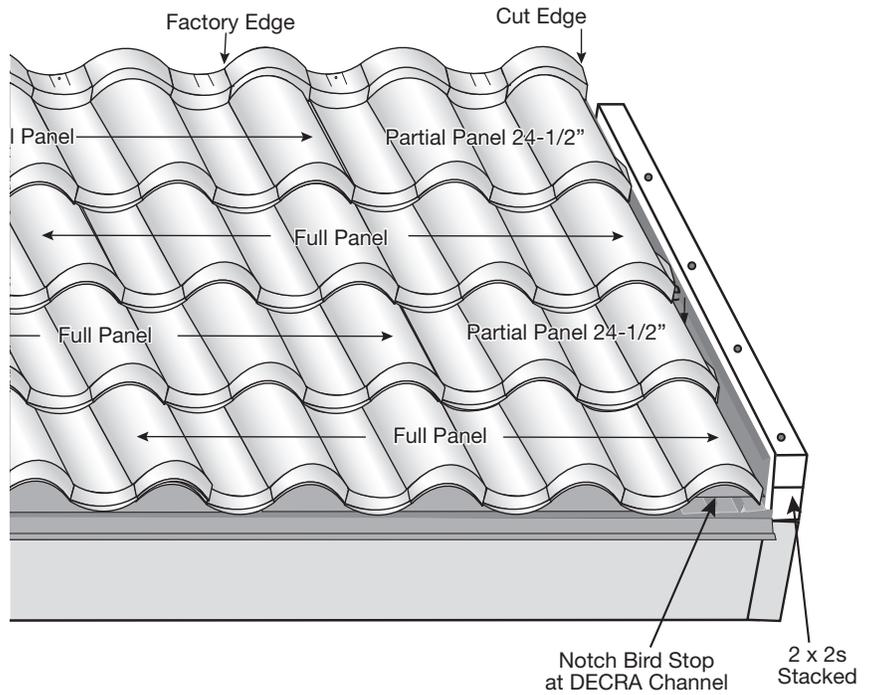
Pre-paint vertical/exposed portion of DECRA Channel & Valley prior to installing panels.
