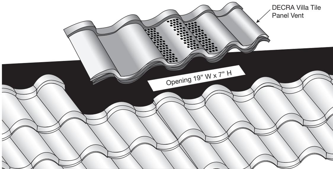
DECRA panel vents should be installed on the last full course below the ridge, and no more than 4 feet down from the peak of the roof facet. Panel vents should NOT be used for air intake.
