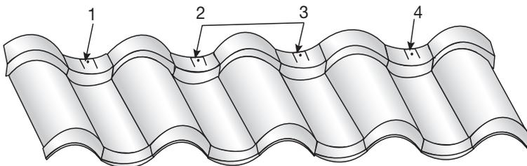
Make sure nose of panel is pulled flush and tight with panel below.
