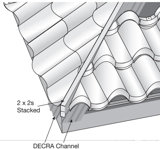
**Panel Installation - Valley:** When installing Villa Panels along the valleys, the panels will terminate into the Villa Valley. See Villa Valley Section (*page 6*) for installation of Villa Valley and preparation prior to installing panels. Measurements for valley cuts are made much like the hip cuts. Measure and cut the panels carefully so they fit tight against the Villa Valley. If a cut-out panel at the valley is too small, lap over two pans to allow proper fastening.
