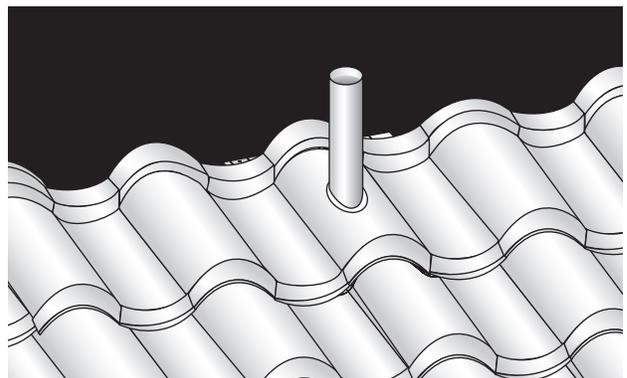
***Do not use LEAD or COPPER with this steel roofing system .***
