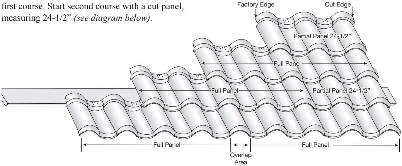
Measure panels and make cuts accordingly so the cut edge starts (or terminates) in the DECRA Channel or Villa Valley (see diagram below). Panels can be cut from either side (see diagram right). Save cut-off pieces for use on opposite side terminating into Villa Valley or DECRA Channel.
