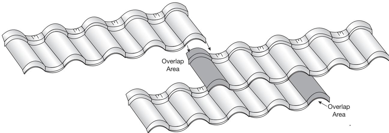
**Fastening Panels - Field:** Attach the second and subsequent courses of panels by locking the front of each panel into the back of the panel below. Fasten each panel to the deck with minimum #9 Hex (1/4" hex head) x 1-1/2" long corrosion resistant screws through the pre-punched fastening tabs along the back of the panels (*see diagram below*).
