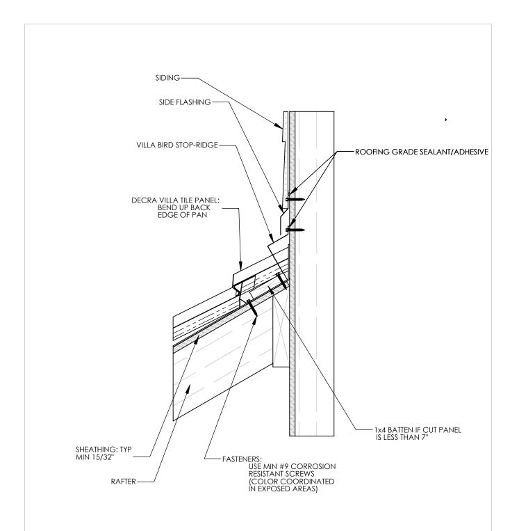
NOTE:FOR BRICK, SEAL THE PANEL BEND TO THE WALL AND COUNTERFLASH WITH SIDE FLASHING
